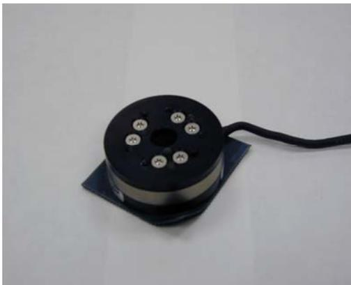
Figure 2 Three-dimensional force transducer used in the study
