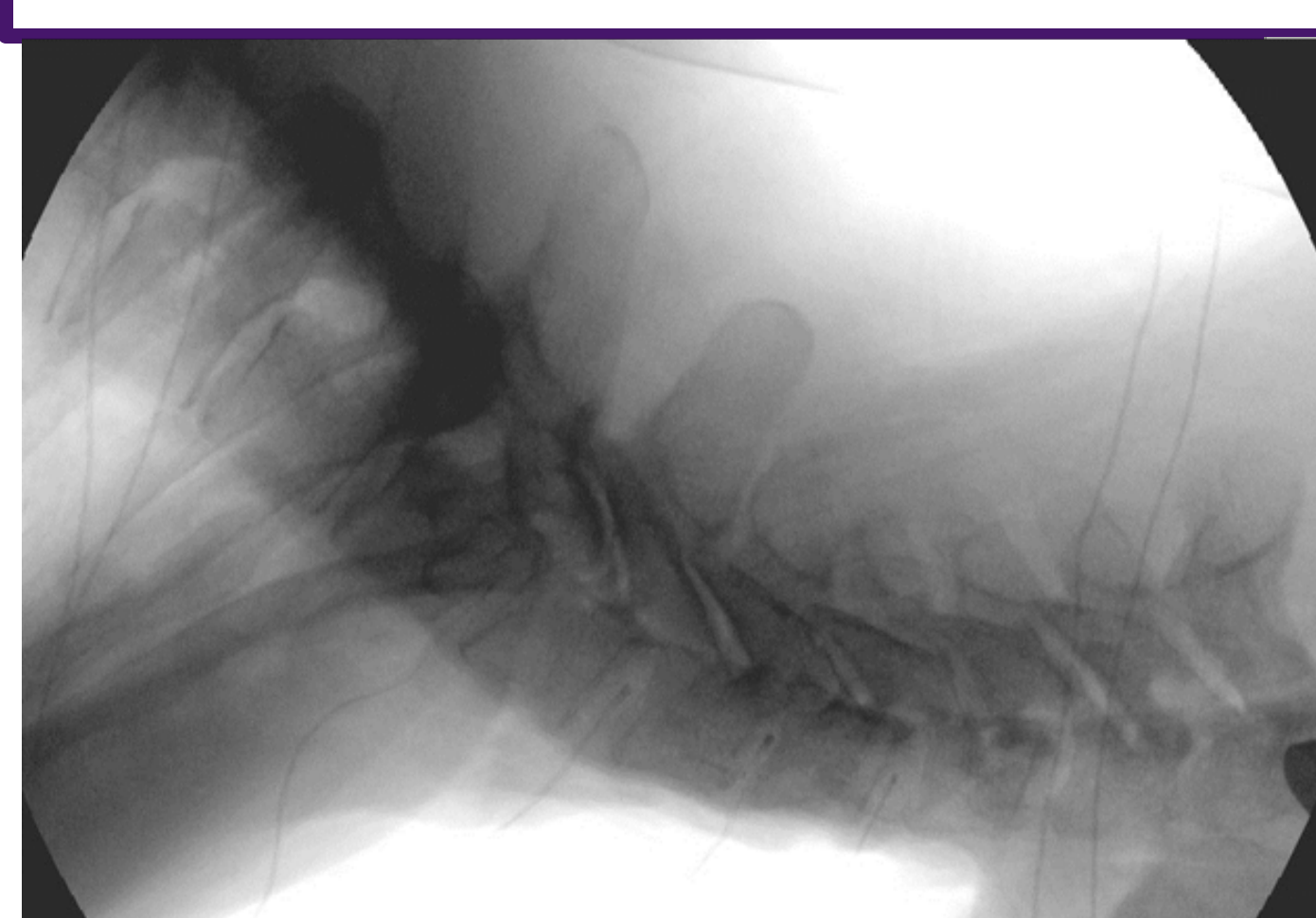
Figure 2. A videofluoroscopic image of the cervical spine with IDP sensors in the nucleus of C4-5, C5-6, C6-7, and C7-T1
